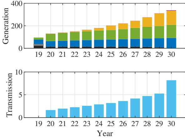
Fig. 5. The optimal generation and transmission capacities [MW]. Fuel oil (black), gas oil (grey), hydro (dark blue), wind (green), solar (yellow), biogas (red), battery (purple) and transmission (light blue).
