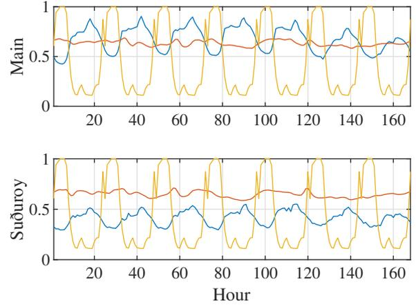
Fig. 4. Example of weekly demand profiles. Regular demand (blue), the heating demand (red) and the electric vehicle demand (yellow).
