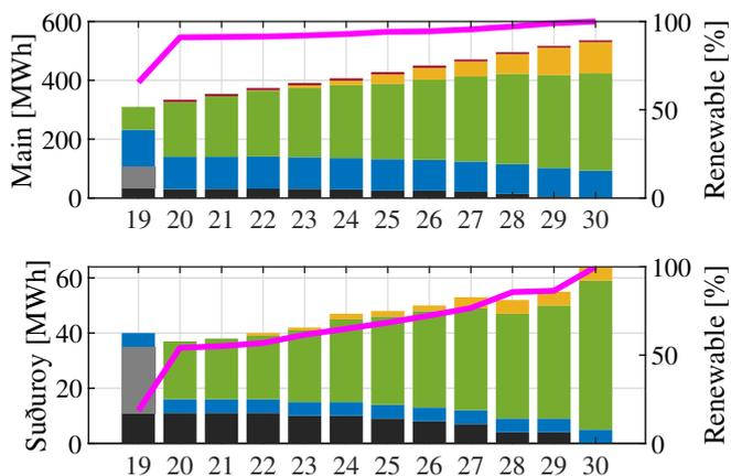
Fig. 7. The optimal production [MWh]. Fuel oil (black), gas oil (grey), hydro (dark blue), wind (green), solar (yellow), biogas (red) and battery (purple).
