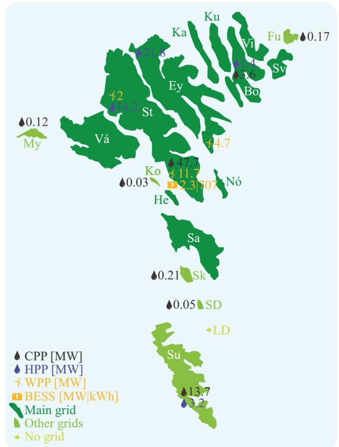
Fig. 1. Overview of the Faroese electrical power grid in 2019. The amounts of installed conventional power plants (CPPs), hydro power plants (HPPs), wind power plants (WPPs), and battery energy storage systems (BESSs) at each site are shown.
