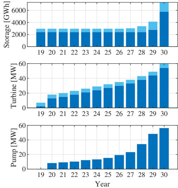
Fig. 6. The storage [MWh], turbine [MW] and pump [MW] capacities for the pumped storage system in the main grid. Upper plant (dark blue) and lower plant (light blue).
