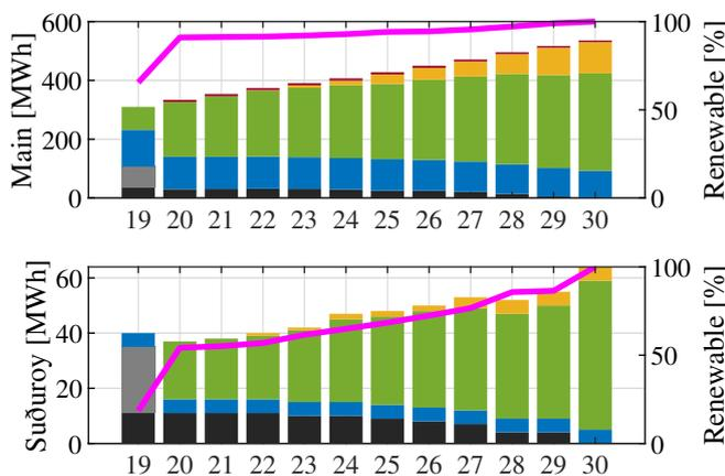
Fig. 7. The optimal production [MWh]. Fuel oil (black), gas oil (grey), hydro (dark blue), wind (green), solar (yellow), biogas (red) and battery (purple).
