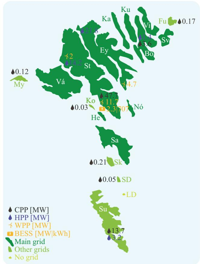
Fig. 1. Overview of the Faroese electrical power grid in 2019. The amounts of installed conventional power plants (CPPs), hydro power plants (HPPs), wind power plants (WPPs), and battery energy storage systems (BESSs) at each site are shown.
