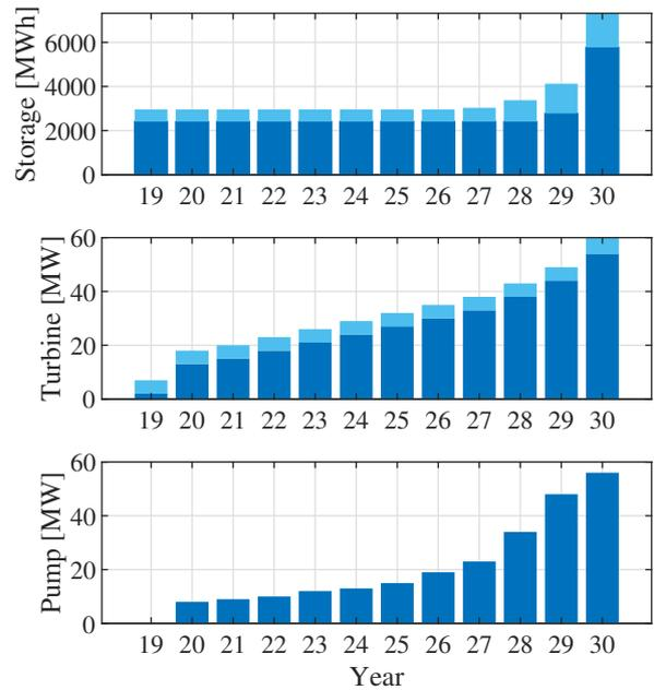
Fig. 6. The storage, turbine and pump capacities for the pumped storage system in the main grid. Upper plant (dark blue) and lower plant (light blue).
